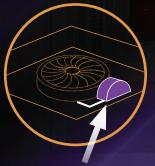
The Elevator Purification Fan system generates negative ions. The ions attach to viruses, bacteria and other microbes, causing a chemical reaction that degrades them.
